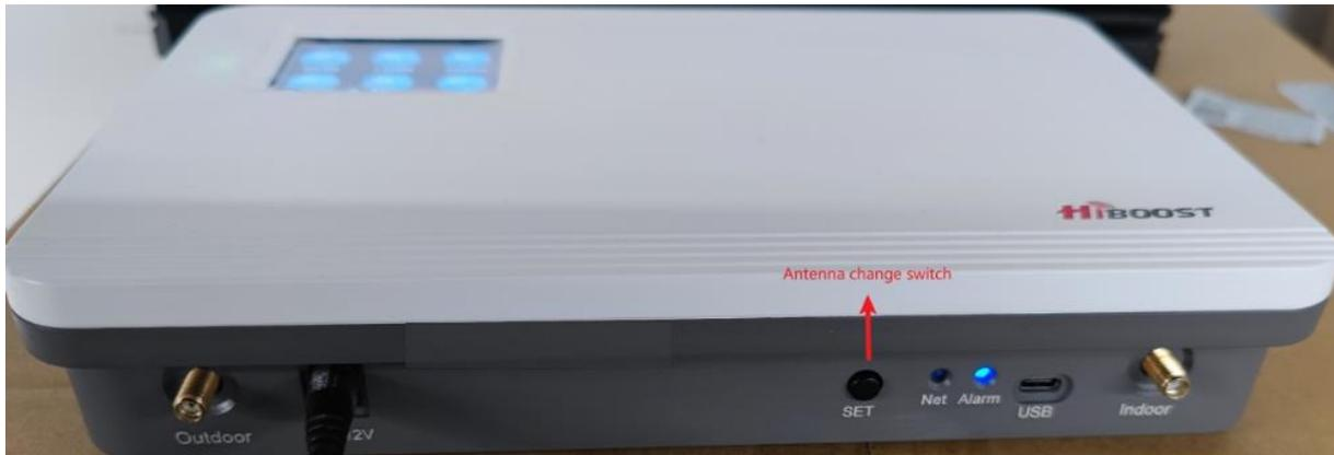
We design one coverage antenna change switch for “SET” button.
