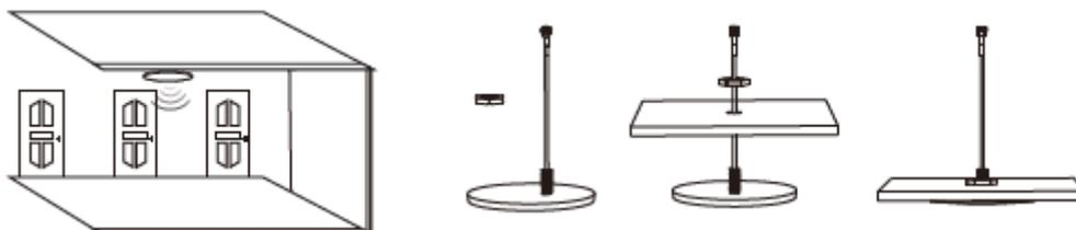
**NOTE:** the required distance between the indoor and outdoor antennas is 10-15 m.
